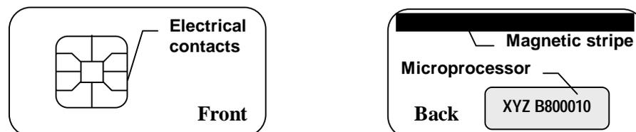
**FIGURE 1-1 Front and Back of Smart Cards**
