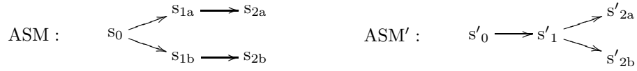
Figure 5: refinement that can be verified with generalized forward simulation, but not with forward simulation
